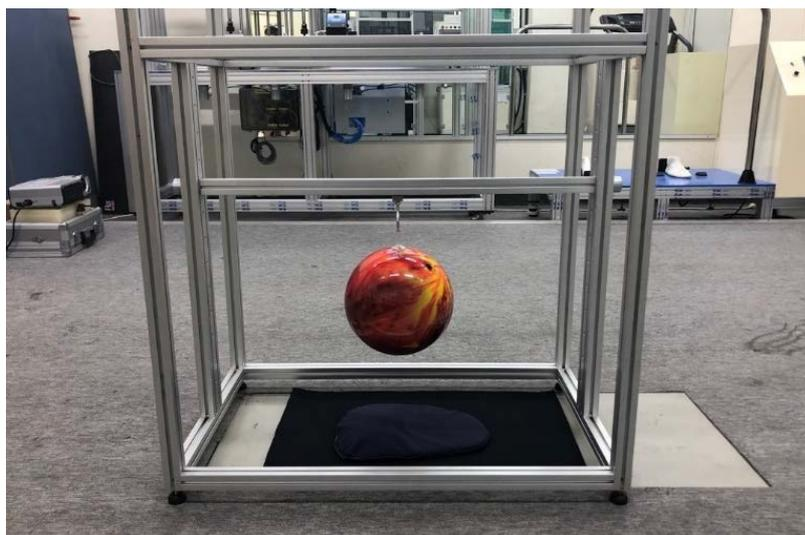
**Figure 6.** Picture of the impact performance test equipment.
