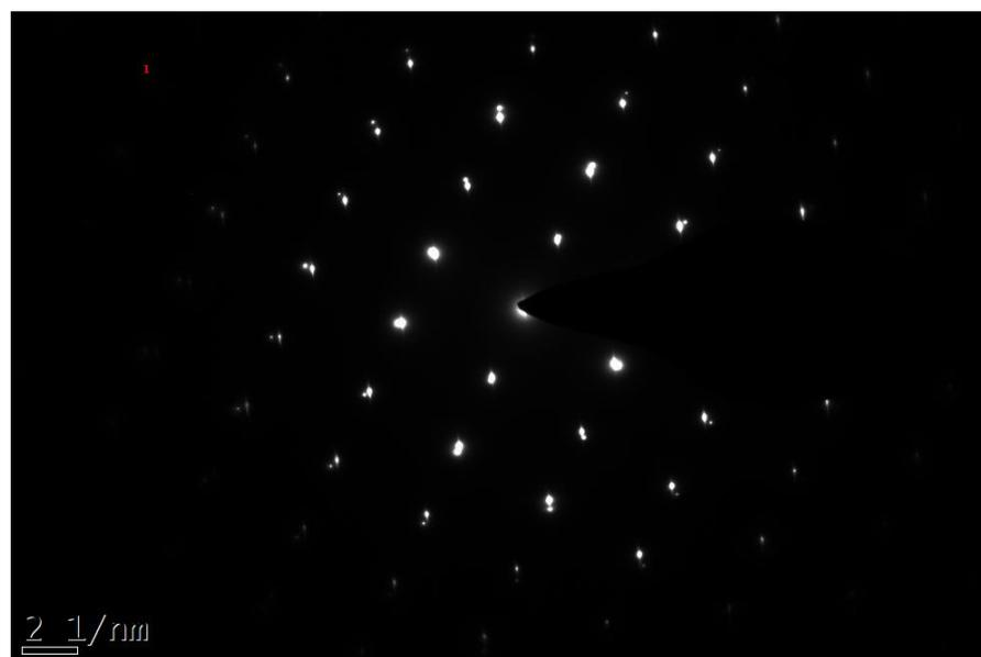
**Figure S1.** TEM images of the sample grown with Air as the carrier gas. (1) Cross-sectional  $\alpha$ - $\text{Ga}_2\text{O}_3$ / $\alpha$ - $\text{Al}_2\text{O}_3$  interface, (2) diffraction spots of  $\alpha$ - $\text{Ga}_2\text{O}_3$ / $\alpha$ - $\text{Al}_2\text{O}_3$ .
