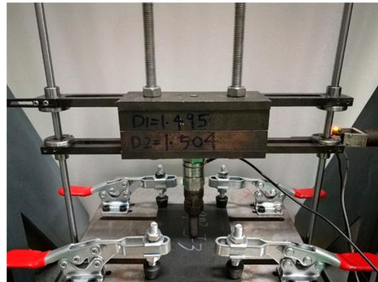
Figure 1. Boundary condition of the impact experiments.
