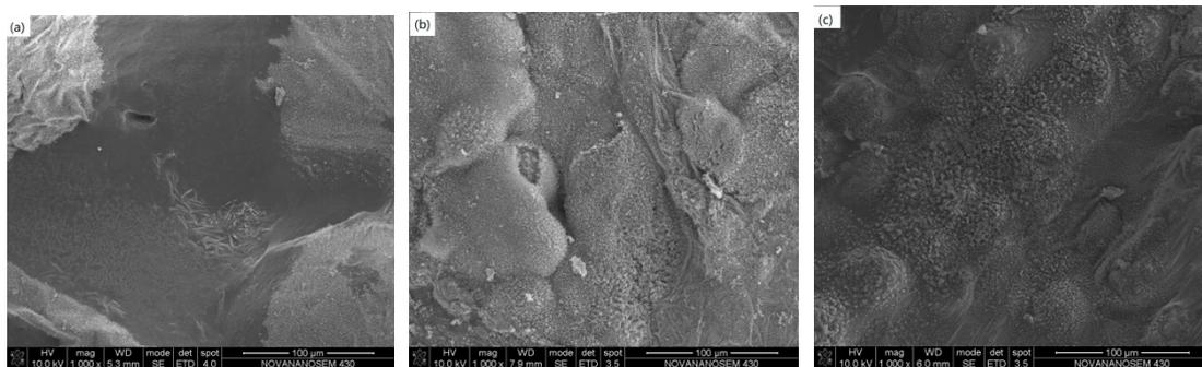
**Figure 5.** SEM photographs of char layer after the UL-94 test of (a) S0, (b) 30% AIN-550RFS, and (c) 50% AIN-550RFS.
