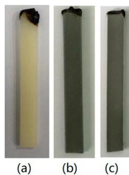
**Figure 3.** Sample morphology photograph after limiting oxygen index (LOI) tests: (a) S0; (b) 30% AIN-550RFS; and (c) 50% AIN-550RFS.
