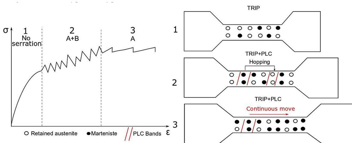
**Figure 2.** The scheme showing the relationship between a serration type and stability of retained austenite in Transformation-Induced Plasticity (TRIP) steels deformed at room temperature.
