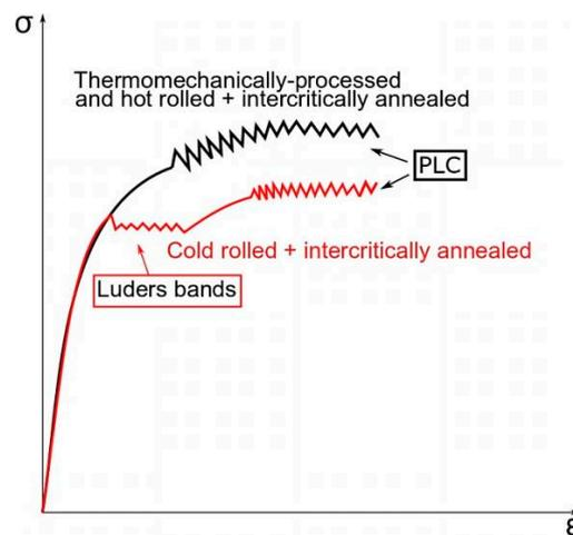
Figure 3. Types of plastic instability in medium-manganese steels.
