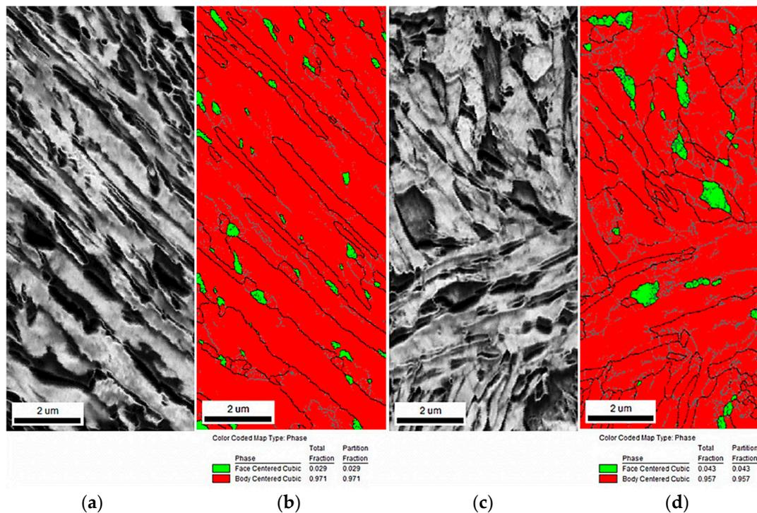
**Figure 5.** Image quality (IQ) maps of the 0.17C–3.1Mn–1.6Al–0.22Si–0.22Mo steel deformed at: 20 °C (a), 140 °C (c) and phase distribution maps obtained at: 20 °C (b), 140 °C (d).
