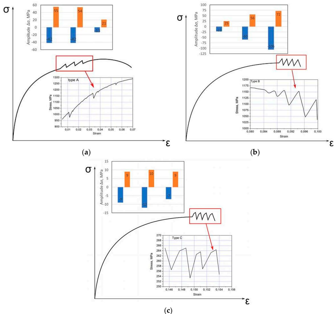
**Figure 1.** Types of oscillations and examples of the histograms of the serration flow: (a) type A, (b) type B and (c) type C.
