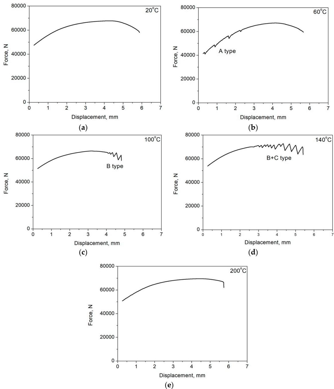
**Figure 4.** Tensile curves of the investigated hot-rolled 0.16C–4.7Mn–1.6Al–0.22Si–0.20Mo steel registered at: (a) 20 °C, (b) 60 °C, (c) 100 °C, (d) 140 °C and (e) 200 °C.
