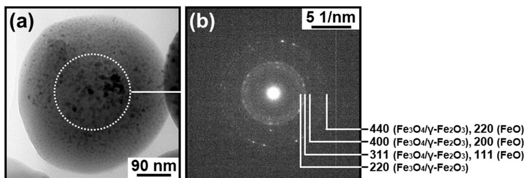
**Figure 7.** (a) TEM image and (b) SAED pattern taken from the white circular area (dotted line) in (a) of the cross-sectional specimen of the type A IO–CaP submicrosphere.
