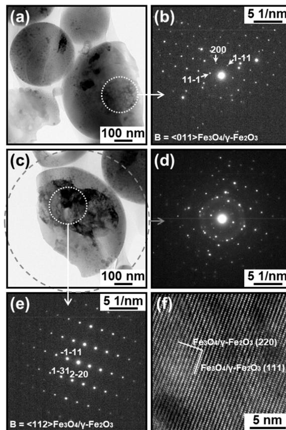
**Figure 8.** (a,c) TEM images, (b,d,e) SAED patterns, and (f) HRTEM image of the cross-sectional specimens of the type B IO–CaP submicrospheres. The SAED patterns in (b,d,e) are taken from the white circular area (dotted line) in (a), the gray circular area (broken line) in (c), and the white circular area (dotted line) in (c), respectively. The HRTEM image is obtained from the white circular area (dotted line) in (c).
