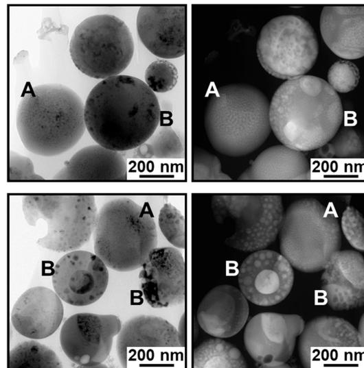
**Figure 3.** TEM (left) and HAADF-STEM (right) images of the representative cross-sectional specimens of the IO–CaP submicrospheres. A: Type A submicrospheres containing single nano-sized (<10 nm) higher density nanoparticles homogeneously dispersed throughout the lower density matrix. B: Type B submicrospheres containing larger higher density nanoparticles, which were mostly a few tens of nanometers (10–100 nm) in size along with one or two submicron-sized (>100 nm) domains.
