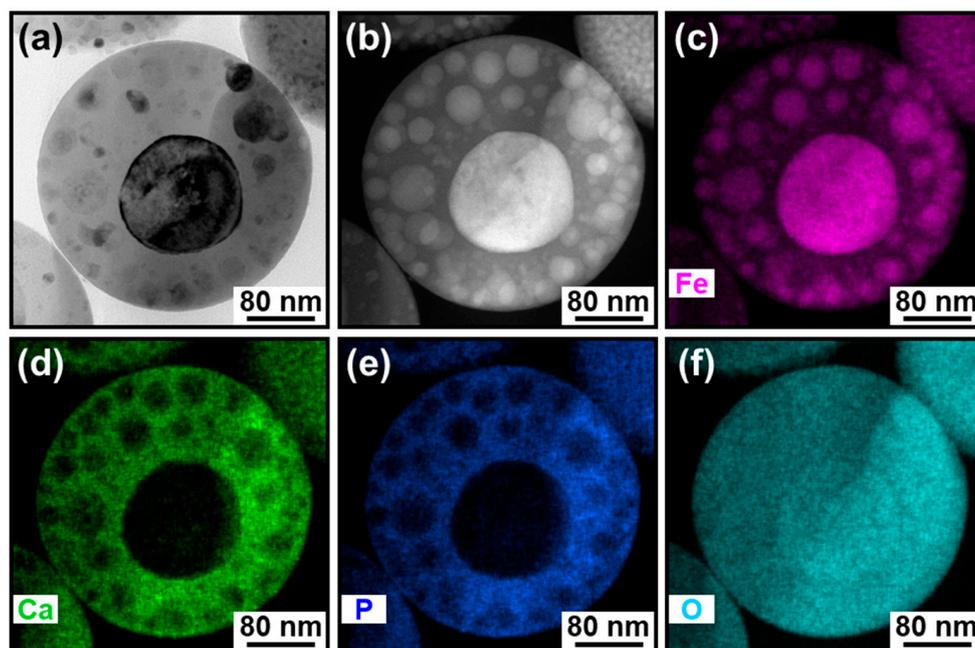
**Figure 6.** (a) TEM and (b) HAADF-STEM images and the elemental distributions of (c) iron, (d) calcium, (e) phosphorus, and (f) oxygen of the cross-sectional specimen of the type B IO–CaP submicrosphere containing spherical IO nanoparticles.
