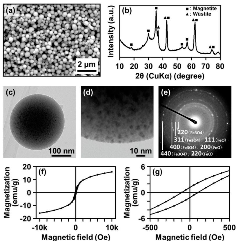
**Figure 1.** (a) SEM image, (b) XRD pattern, (c,d) TEM images (whole picture (c) and outer region (d)), (e) TED image, and (f,g) magnetization curves at 300 K ((g) is the magnified curve around the origin) of the IO–CaP submicrospheres (reproduced from [18] with permission from the PCCP Owner Societies).
