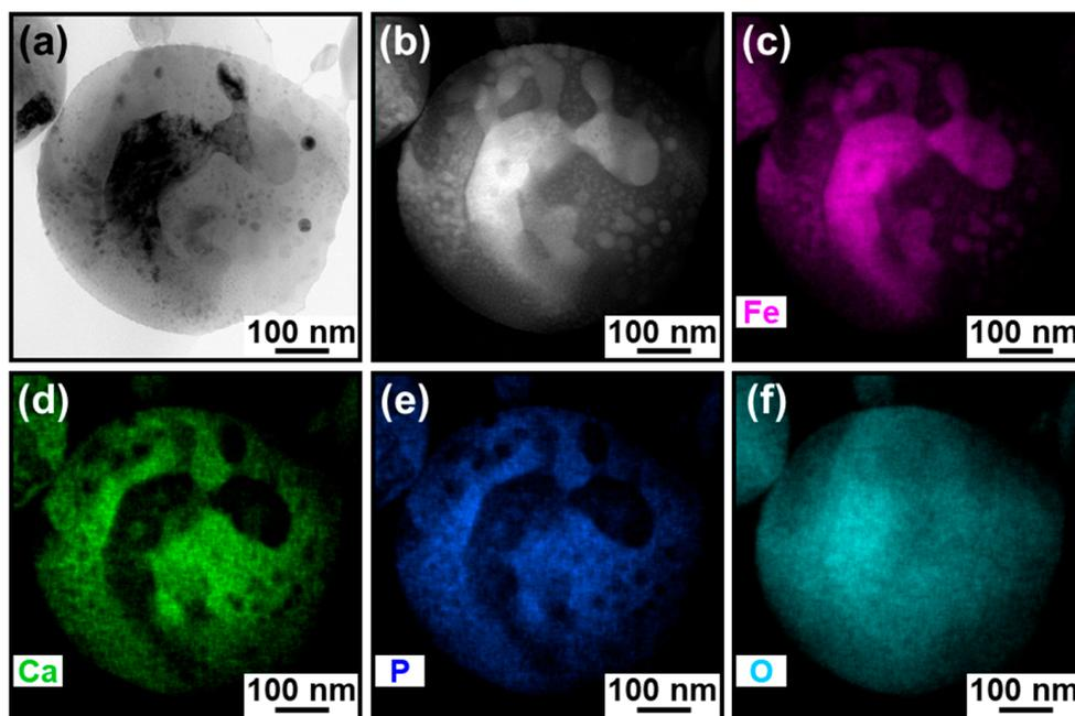
**Figure 5.** (a) TEM and (b) HAADF-STEM images and the elemental distributions of (c) iron, (d) calcium, (e) phosphorus, and (f) oxygen of the cross-sectional specimen of the type B IO–CaP submicrosphere containing irregularly-shaped IO nanoparticles.
