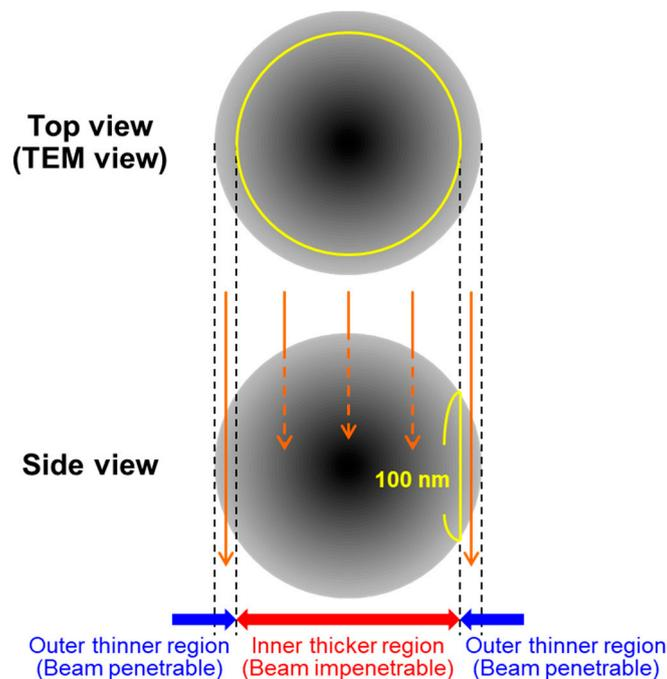
**Figure 2.** Schematic illustration of the outer thinner region and the inner thicker region of the submicrosphere.
