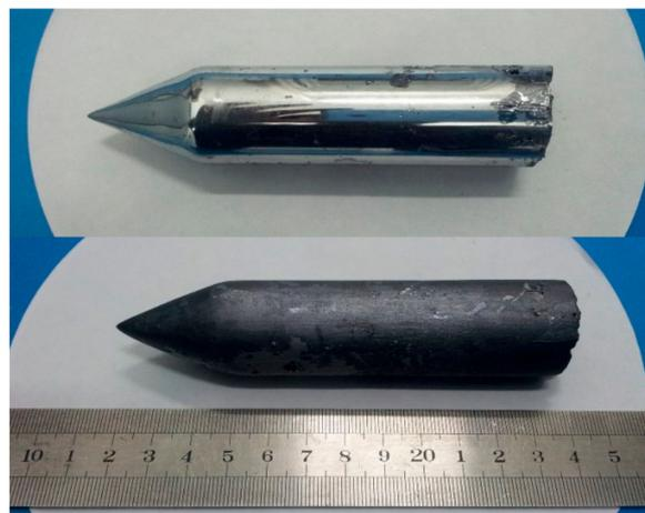
**Figure 1.** Picture of the cadmium–magnesium–telluride (CdMgTe) ingot grown by the modified vertical Bridgman method.
