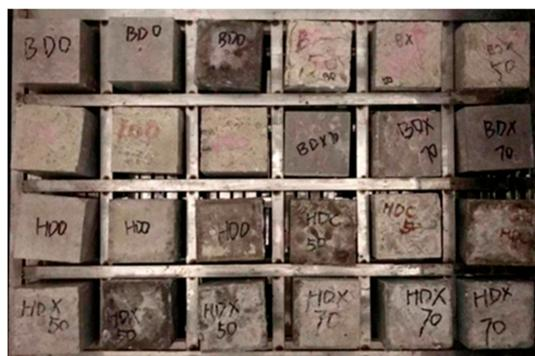
**Figure 3.** Carbonation testing.
