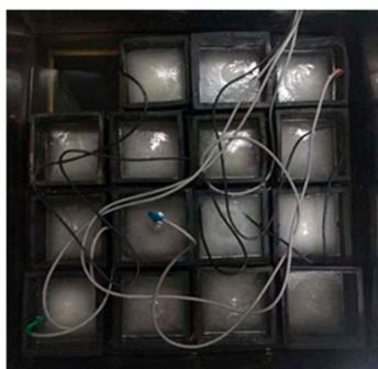
**Figure 2.** Freezing and thawing testing.
