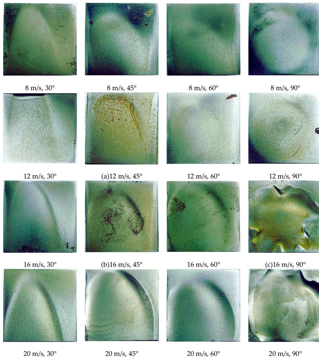
**Figure 11.** Surface images of 13Cr after erosion and corrosion in liquid–solid two-phase flow.
