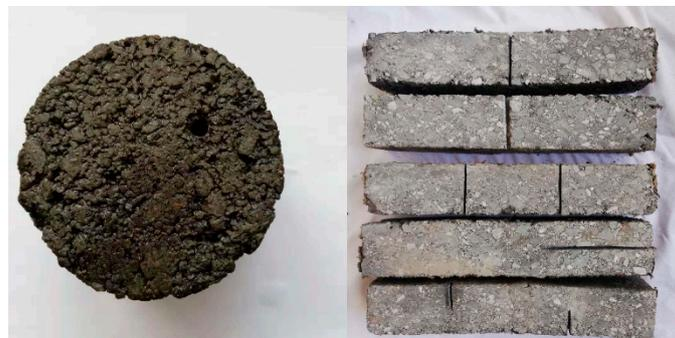
**Figure 1.** The factitious damage of specimens.
