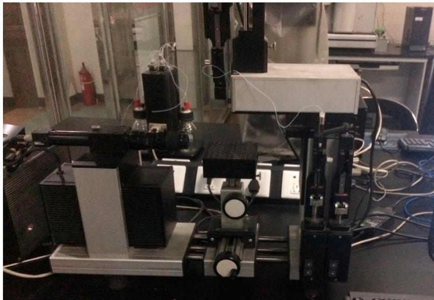
Figure 10. Optical video contact angle tester (OCA20).
