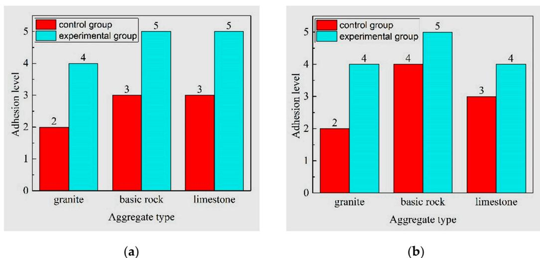
**Figure 4.** Asphalt-aggregate adhesion level based on stripping test: (a) #90 asphalt and (b) #110 asphalt (samples without treated were marked as control group, while the ones soaked with plant ash lixivium were marked as experimental group).
