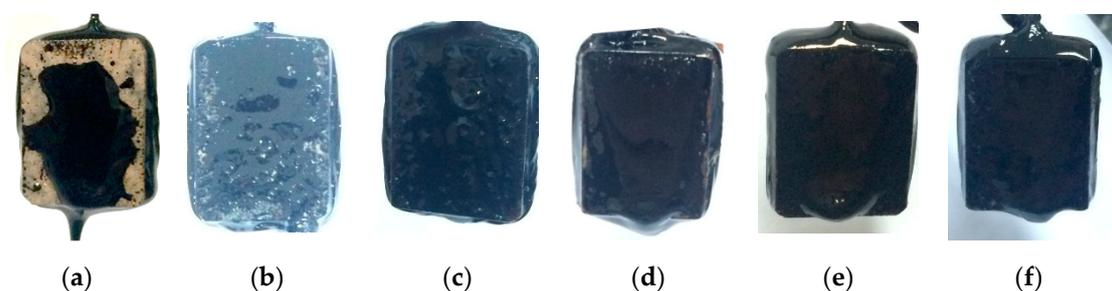
**Figure 6.** The specimens after modified stripping test: (a–c) control specimens with granite, basic rock, and limestone and (d–f) treated specimens with granite, basic rock, and limestone.
