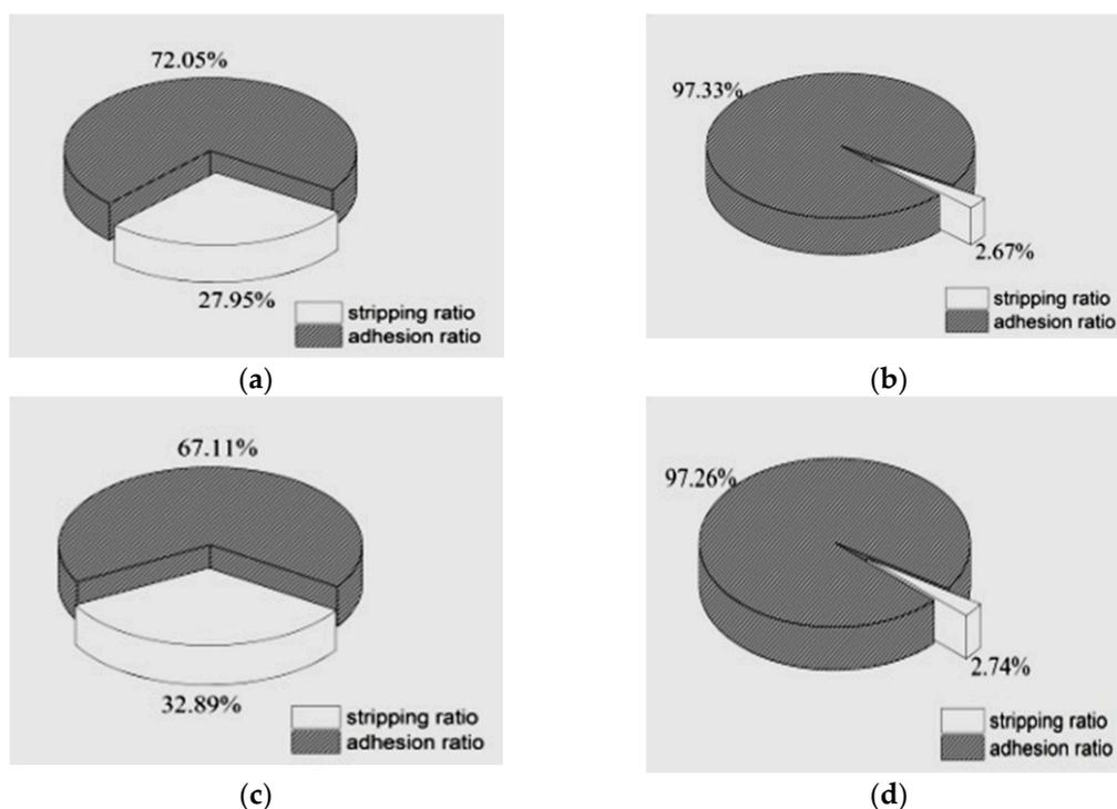
**Figure 9.** The adhesion and stripping ratios of granite specimen after modified stripping test: (a) control specimen with #90 asphalt; (b) treated specimen with #90 asphalt; (c) control specimen with #110 asphalt; and (d) treated specimen with #110 asphalt.
