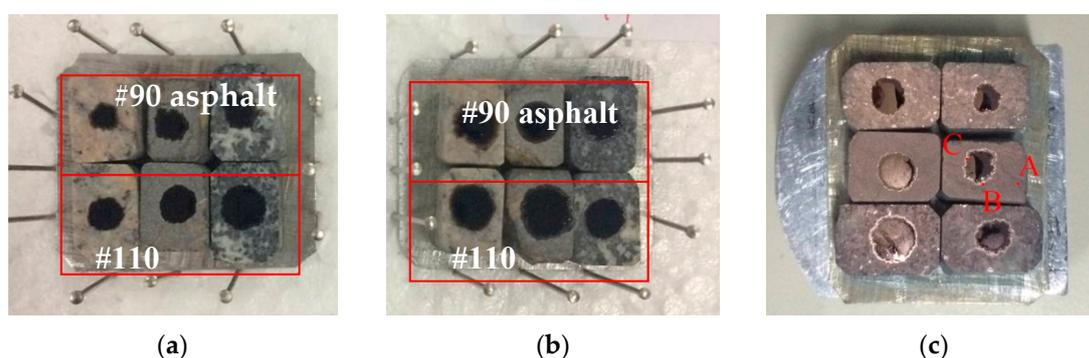
**Figure 12.** Specimens for scanning electron microscopy (SEM) with energy dispersive spectroscopy (EDS) measurements: (a) control; (b) treated specimen; and (c) observation locations at one specimen (A, B, C).
