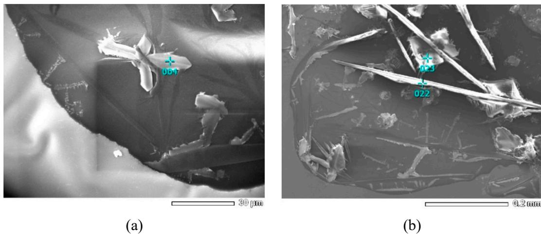
**Figure 14.** Observed crystal substances: (a) feather-like and (b) needle-like and square shape.
