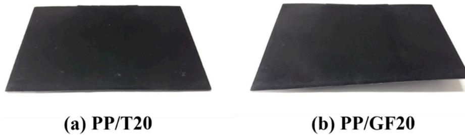
**Figure 8.** Warpage of test samples: (a) PP/T20 and (b) PP/GF20.
