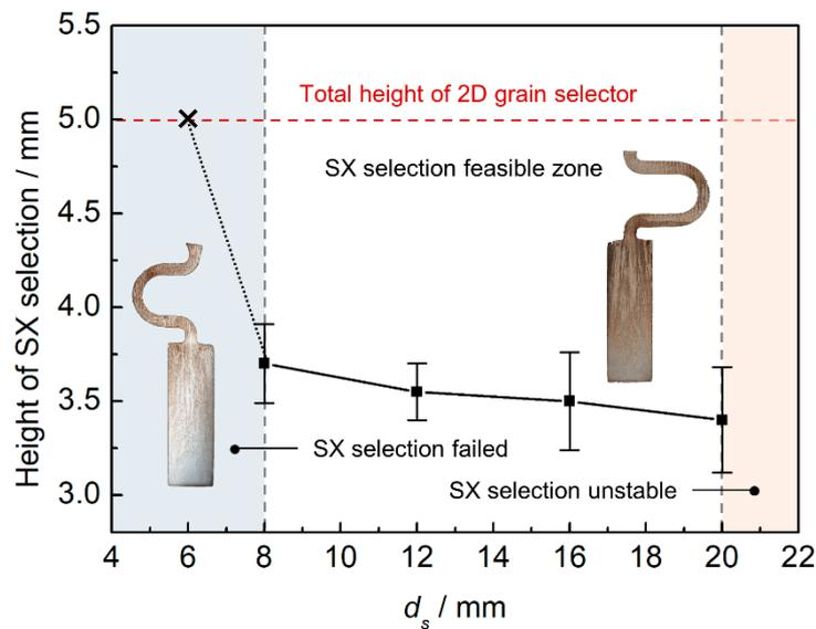
**Figure 6.** The relationship between heights of SX position and selector eccentric distance ( $d_s$ ).
