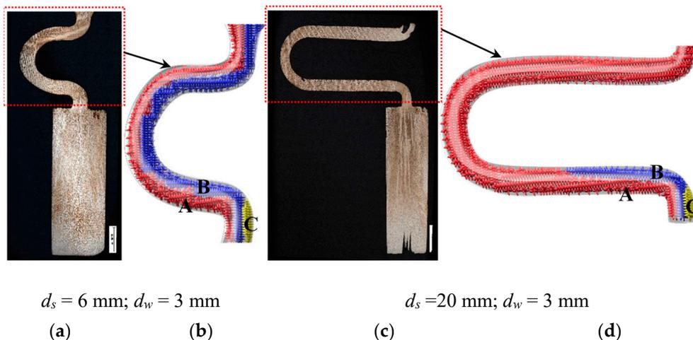
**Figure 7.** Optical images of the dendrite structure in the selector parts of the selectors with 3 mm (a) and 20 mm (c) eccentric distance as well as their corresponding schematic diagrams (b) and (d).
