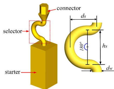
**Figure 1.** Schematic drawings of the new 2D grain selector and its selector part showing parameters used in the selector part.
