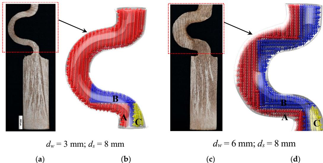
Figure 5. Optical images of the dendrite structure in the selector parts of the selectors with 3 mm (a) and 6 mm (c) thickness as well as their corresponding schematic diagrams (b) and (d).
