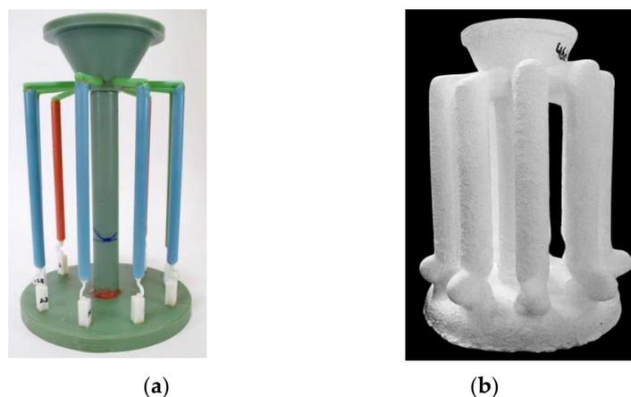
**Figure 2.** Images of the wax model (a) and the shell mold (b).
