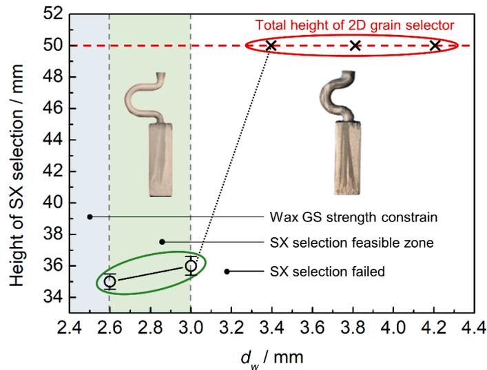
Figure 4. Experimentally observed heights of SX position versus selector thickness ( $d_w$ ).
