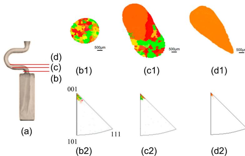
**Figure 3.** Optical image of the selector part of the 2D grain selector having 3 mm thickness and 8 mm eccentric distance (a); EBSD IPF-X maps on the grain structure evolution (b1,c1,d1) and the EBSD inverse pole figures in growth direction at different heights (b2,c2,d2).
