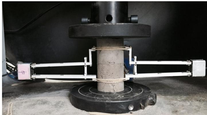
Figure 7. Compressive test of ECC.
