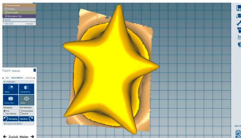
Figure 6. Star-shaped zirconia crown designing using Ceramill Mind software (Amann Girrbach).
