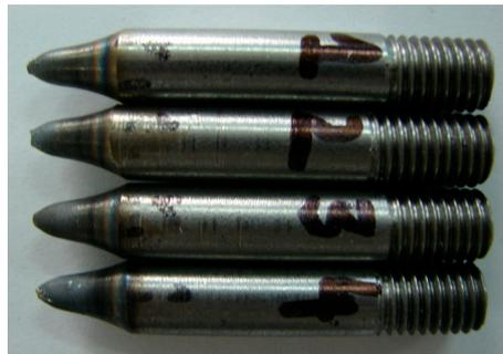
**Figure 5.** R200 steel specimens fractured in the tensile test performed with the Gleeble 3800 simulator at a temperature range of 1–900 °C (this temperature range was excluded from the fracture analysis since the plastometric test was constrained to the temperature range of 1000 °C–200 °C), 2–1000 °C, 3–1100 °C, and 4–1200 °C.
