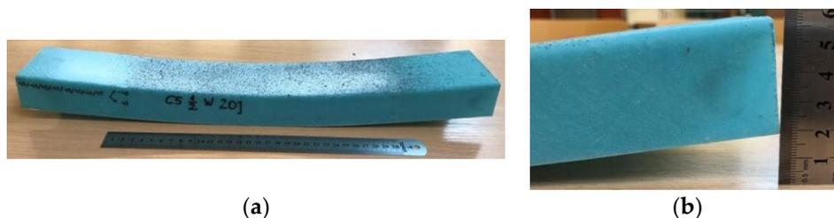
**Figure 6.** Permanent (a) “plastic” deflection in unloaded Cb5 beam with zoom view (b).
