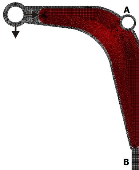
**Figure 26.** The control arm: The design domain, loads and supports.
