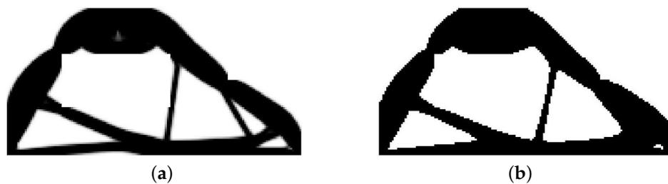
**Figure 22.** The generation of minimal compliance topologies for test structure 4. (a) The final topology using Algorithm (1). (b) The final topology using Algorithm (2).
