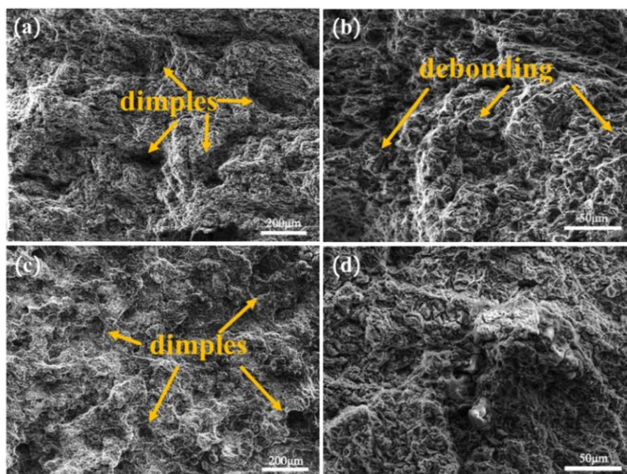
**Figure 7.** Low- (a,c) and high- (b,d) magnification SEM images of 5% Grp/AZ91 composites after hot deformation: 1FD (a,b); 1FD+ED (c,d).
