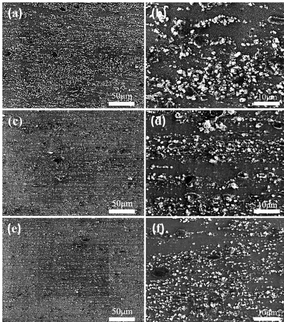
**Figure 6.** Low- (a,c,e) and high- (b,d,f) magnification SEM images of 5% Grp/AZ91 composites fabricated by multistep deformation: 1FD+ED (a,b); 3FD+ED (c,d); 6FD+ED (e,f).
