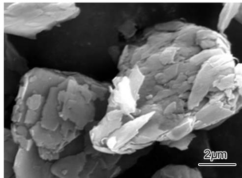
**Figure 1.** SEM image of particle morphology for Grp.
