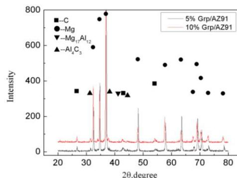
**Figure 4.** The X-ray diffraction of the as-cast Grp/AZ91 composites.
