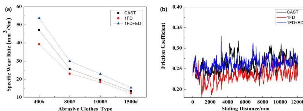
**Figure 9.** (a) Wear rate under different cloth abrasiveness types, and (b) friction coefficient versus time of the 5% Grp/AZ91 composites after hot deformation.
