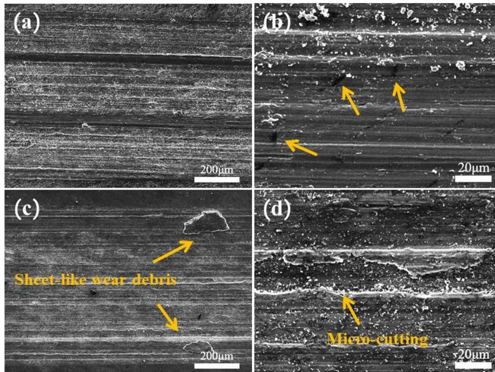
**Figure 10.** Low- (a,c) and high- (b,d) magnification SEM images of the worn surface of the 5% Grp/AZ91 composites after hot deformation: 1FD (a,b); 1FD+ED (c,d).
