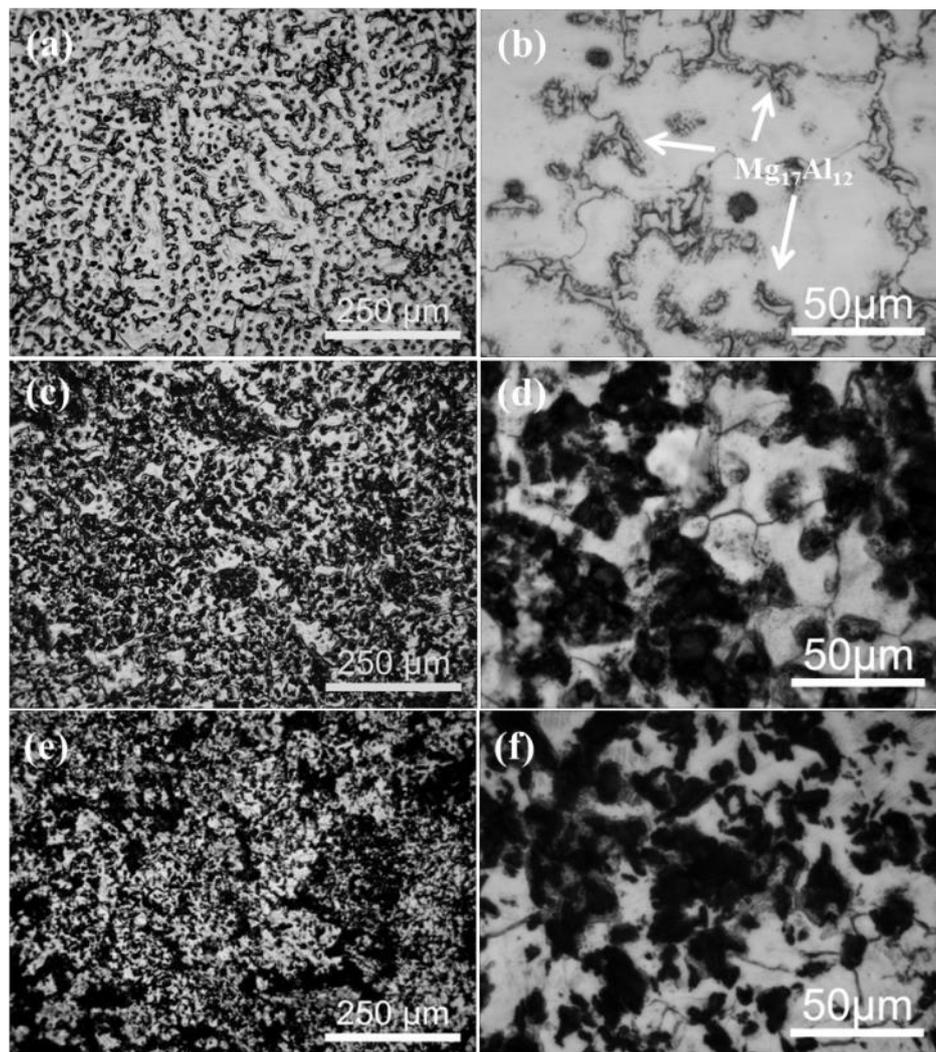
**Figure 2.** Low- (a,c,e) and high- (b,d,f) magnification OM images of the as-cast Grp/AZ91 composites: AZ91 alloy (a,b); 5% Grp/AZ91 composites (c,d); 10% Grp/AZ91 composites (e,f).
