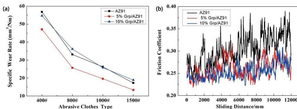
**Figure 8.** (a) Wear rate with different abrasive cloths, and (b) the friction coefficient versus time of the as-cast AZ91 alloy and Grp/AZ91 composites.
