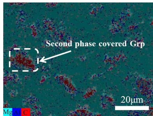
**Figure 3.** EDS of as-cast 5% Grp/AZ91 composites.
