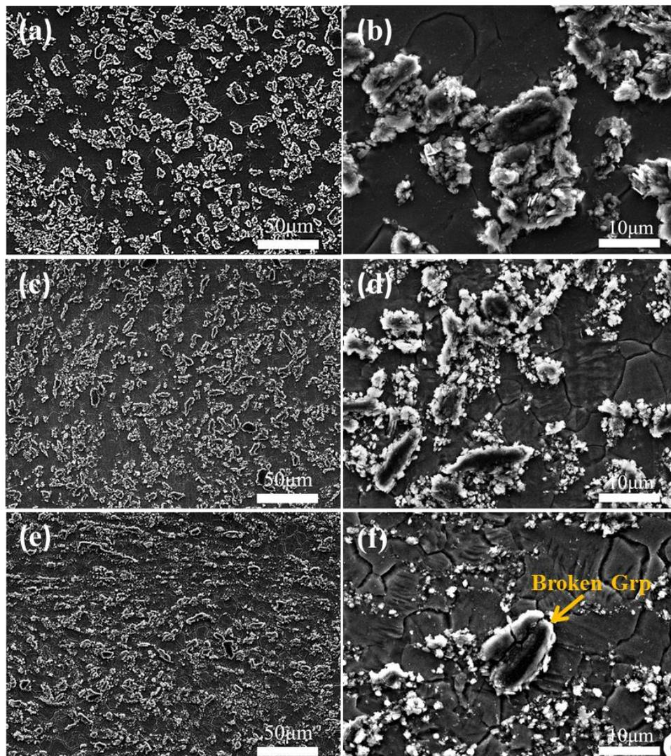
**Figure 5.** Low- (a,c,e) and high- (b,d,f) magnification SEM images of 5% Grp/AZ91 after MDF: 1FD (a,b); 3FD (c,d); 6FD (e,f).
