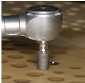
**Figure 1.** Implant placement in dense bone simulant.
