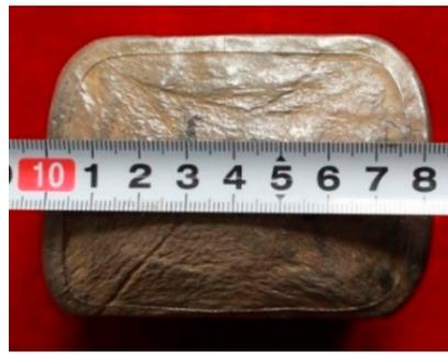
**Figure 6.** External appearance of Ti-43Al-2Cr-1.5Mn-0.2Y alloy fabricated by MDF with a reduction of 30% per pass.
