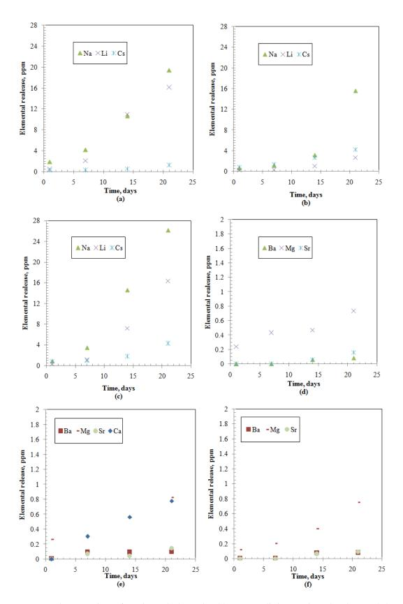
**Figure 1.** Elements releases from the studied samples: (a) Group I-Alkali-Borosilicate (ABS)-Waste (17); (b) Group I-Modified Alkali-Borosilicate (MABS)-Waste (20); (c) Group I-ABS-Waste (25); (d) Group II-ABS-Waste (17); (e) Group II-MABS- Waste (20); (f) Group II-ABS-Waste (25).
