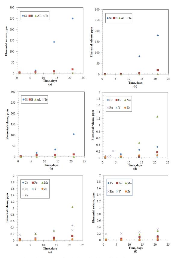
**Figure 2.** Elemental releases from the studied samples: (a) Metalloid and post-transition-ABS-Waste (17); (b) Metalloid and post-transition-MABS-Waste (20); (c) Metalloid and post-transition-ABS-Waste (25); (d) Transition-ABS-Waste (17); (e) Transition-MABS-Waste (20); (f) Transition-ABS-Waste (25).
