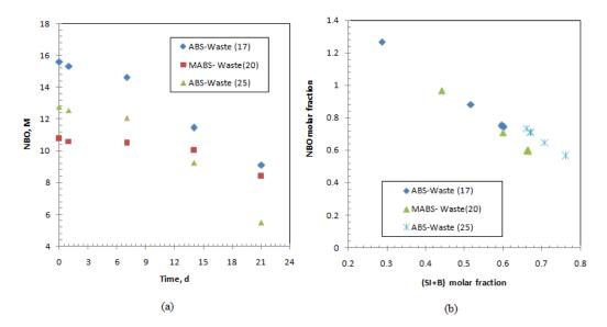
**Figure 4.** The evolution of glass matrix composition during the leaching process: (a) temporal changes in non-bridging oxygen (NBO); (b) The NBO fraction as a function of former fraction.
