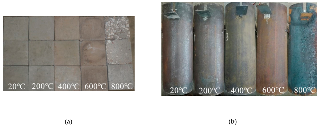
Figure 5. Appearance of specimens after water-cooling. (a) high strength concrete test blocks; (b) specimens.
