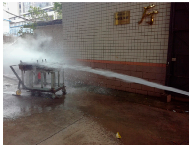
Figure 3. Specimens cooled by fire hydrant after high temperatures exposure.
