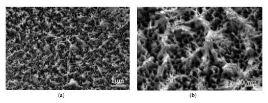
Figure 7. The microstructures of the anodized aluminum alloys surface: (a) ×10,000, (b) ×30,000.
