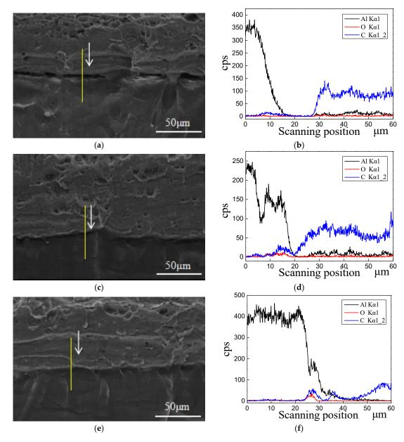
**Figure 9.** The SEM photos of the cross sections of UAHPT samples: (**a**) No.1, (**c**) No.8, (**e**) Optimum processed sample; the line scan chemical analysis at the interfaces of samples: (**b**) No.1, (**d**) No.8, and (**f**) Optimum processed sample.
