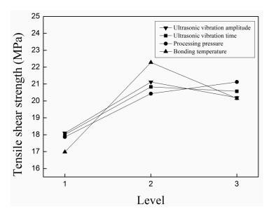
Figure 3. The tensile shear strengths versus UAHPT processing variables.
