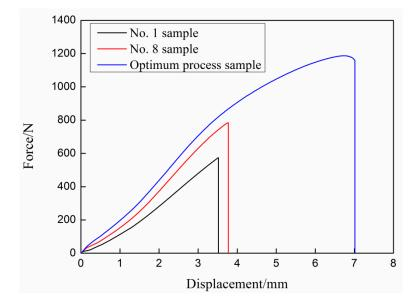
Figure 4. The typical load-displacement curves of the UAHPT prepared specimens.
