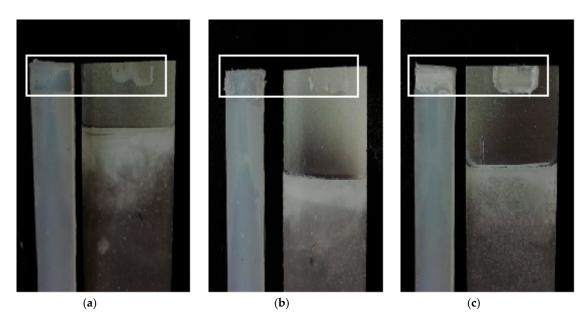
**Figure 5.** Fracture failure photos of different UAHPT specimens: (**a**) No. 1 sample, (**b**) No. 8 sample, and (**c**) Optimum processed sample.
