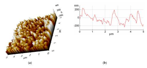
**Figure 8.** The AFM topography of the anodized aluminum alloy surface: (**a**) atomic force morphology, (**b**) hole depth.
