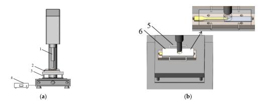
**Figure 1.** The experimental device for the ultrasonic assisted hot-pressing technology: (**a**) ultrasonic welding machine (1-ultrasound vibration press head, 2-mold, 3-heating table, 4-controller); (**b**) mold diagram (5-adiabatic handle, 6-pressed steel plate).
