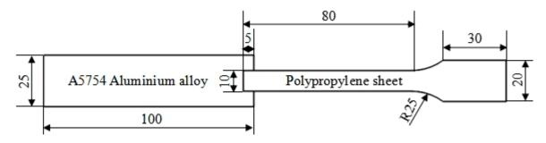
Figure 2. The sketch diagram of single-lap of polypropylene/aluminum alloy hybrid.
