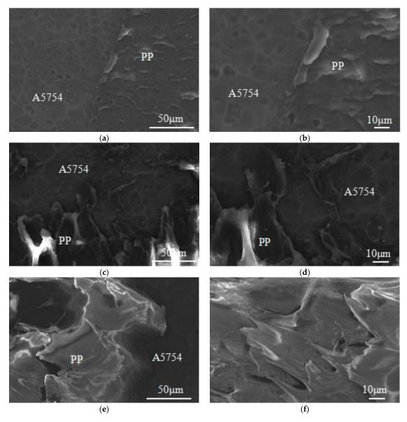
**Figure 6.** SEM photos of the UAHPT samples after tensile shear test: (**a**) and (**b**) NO.1sample, (**c**) and (**d**) NO.8 sample, (**e**) and (**f**) Optimum processed sample.
