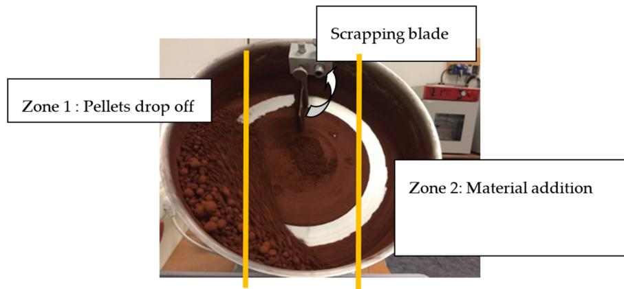
**Figure 1.** Illustration of the granulation process.
