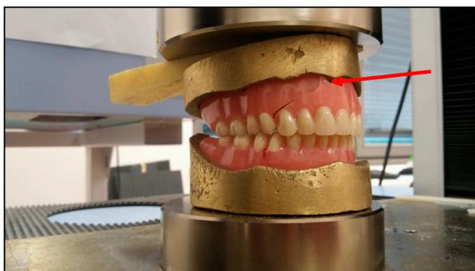
**Figure 5.** Tooth denture PMMA/ZnO NPs after the compressive testing and the place where the crack started (red arrow).
