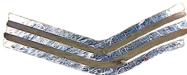
Figure 23. Failure mode after short-beam three-point-bending test with a span-to-thickness ratio of 4.
