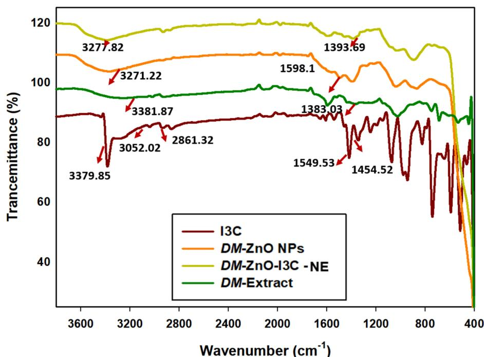
**Figure 3.** Fourier transforms infrared analysis (FTIR) for I3C standard (Red), DM-ZnO NPs (orange) DM-ZnO-I3C-NE (yellow) and DM extract (green).
