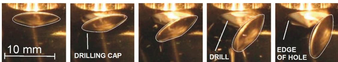
Figure 14. Camera frames showing subsequent stages of drilling with a factory drill.
