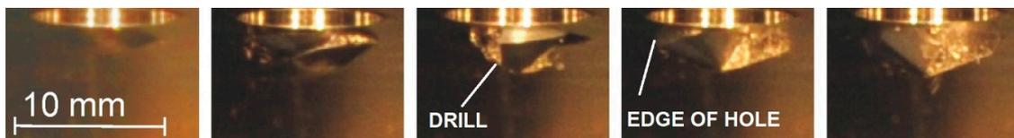
Figure 15. Camera frames showing subsequent stages of drilling with a modified drill.
