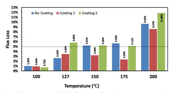
Figure 5. Temperature variation of the flux-loss% over 1000 h annealing at various temperatures with and without protective resin coating to mimic the permanent magnet operation cycle. Magnetized bonded magnets were coated with  $\sim \! 10~\mu m$  thick protective resin coatings (3M Scotch-Weld DP100 (designated as coating #1) and J-B Weld epoxy coating (designated as coating #2)).
