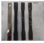
**Figure 6.** Tensile stress-displacement curve of the Big Area Additive Manufacturing (BAAM) fabricated NdFeB PPS magnets (**left**); Fractured dog-bone shaped magnets after tensile evaluation (**right**).
