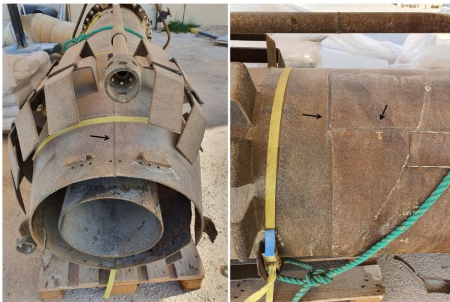
**Figure 11.** Longitudinal and circumferential welding line in the flare body part.
