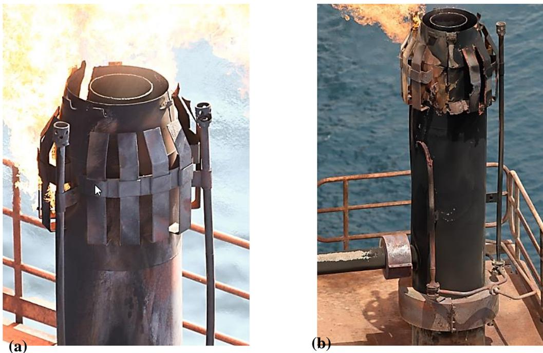
Figure 2. The investigated Gas flare Tip (a) Gas fare tip (b) Gas flare tip with immature failure.
