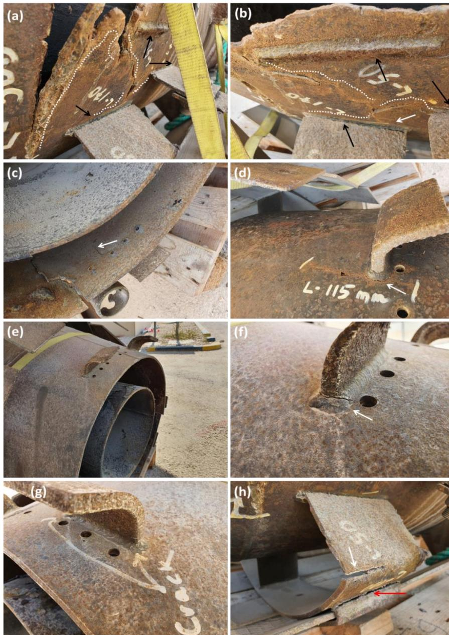
**Figure 12.** A detailed study of the root cause of the failure region in the vicinity of the joints (a–c,f,h) The most critical sections that failure took place (d,g) welding at the vicinity of holes (e) the upper part of the flare tip.
