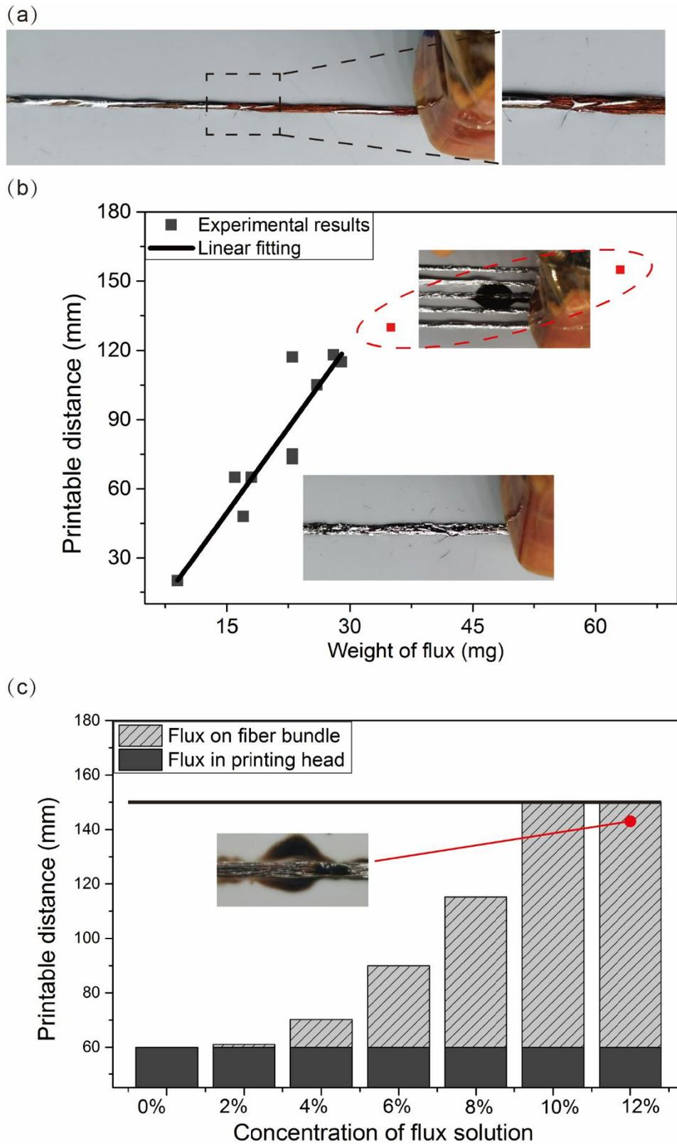
**Figure S1.** (a) The image of Cu-CF/Pb50Sn50 printed without flux; (b) The printable distances varied with the weights of flux inside the printing head; (c) The printable distances varied with the concentrations of flux solution.
