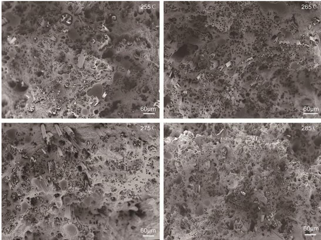
**Figure S2.** Morphologies of fracture surface for composite specimens at different temperatures.
