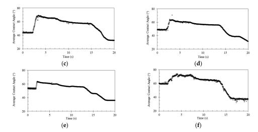
**Figure 7.** Changes of the water contact angles of the Ti6Al4V surface coated with (**a**) pDA, (**b**) pDA-KR12, (**c**) pDA-KR12/32, (**d**) pDA-KR12-5911, (**e**) pDA-KR12/32-5911, and (**f**) Ti6Al4V without coating, showing the changes in the water droplet's volume.
