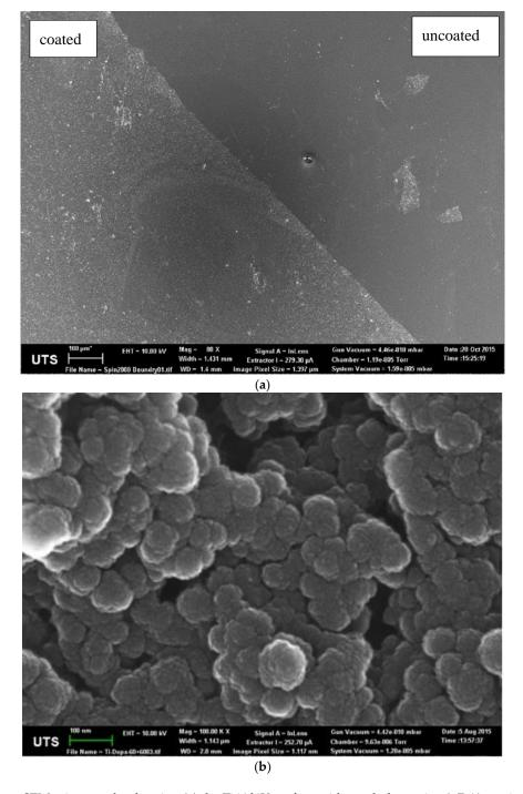
**Figure 3.** SEM micrographs showing (**a**) the Ti6Al4V surface with a polydopamine (pDA) coating (left) and uncoated (right) at a magnification of  $1000\times$ , as well as (**b**) the pDA coating at  $100,000\times$  magnification.
