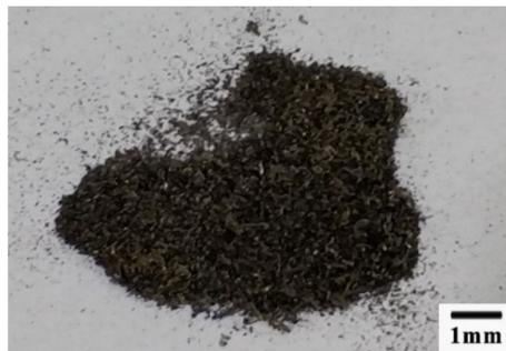
**Figure 23.** The chips formed when the cutting speed was above 600 m/min.
