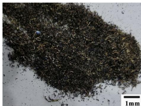
**Figure 24.** The chips formed when the cutting speed was below 600 m/min.
