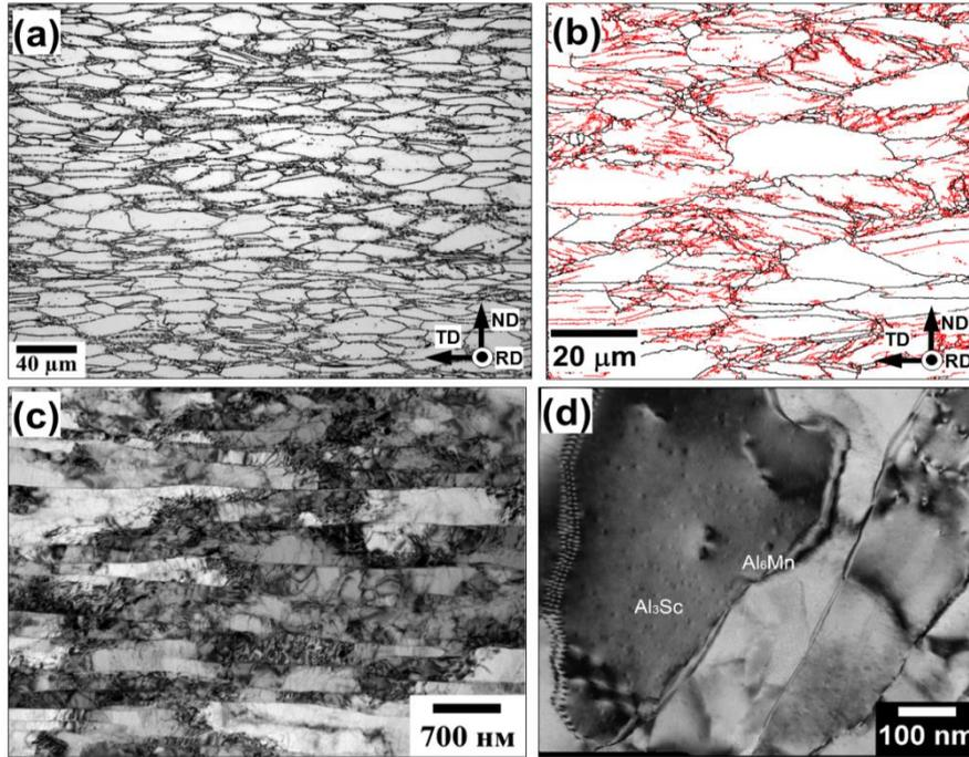
**Figure S2.** Initial microstructure of the hot-rolled Al-Mg-Sc alloy: optical micrograph (a), EBSD grain-boundary map (b) and TEM images (c), (d). In (b), low- and high-angle boundaries are depicted as red and black lines, respectively.
