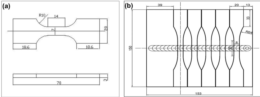
**Figure S4.** Design of the fatigue specimens machined from the welded sheets of Al-Mg-Sc alloy (a) and 6061 alloy (b). In all cases, units are mm. Not in scale.
