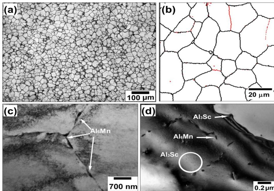
**Figure S1.** Initial microstructure of the cast Al-Mg-Sc alloy: optical micrograph (a), EBSD grain-boundary map (b) and TEM images (c, d). In (b), low- and high-angle boundaries are depicted as red and black lines, respectively.
