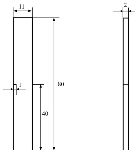
**Figure 3.** The single edge-cracked tension specimen for fatigue tensile test (unit: mm).
