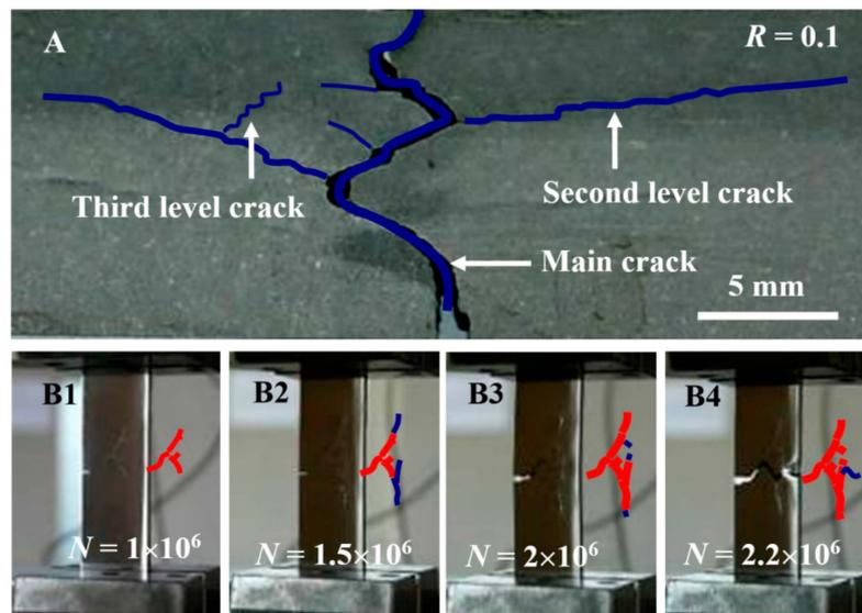
**Figure 6.** Extreme damage tolerance in tension–tension fatigue test. (A) Image of three-level fatigue cracks. (B1–B4) Crack propagations with cycle numbers  $N$ , in which the red and blue curves demonstrate the existing cracks in the former image and the extended cracks respectively.
