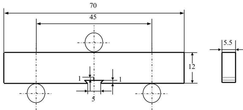
**Figure 2.** The single edge-cracked bend specimen for the three-point bending fatigue test (unit: mm).
