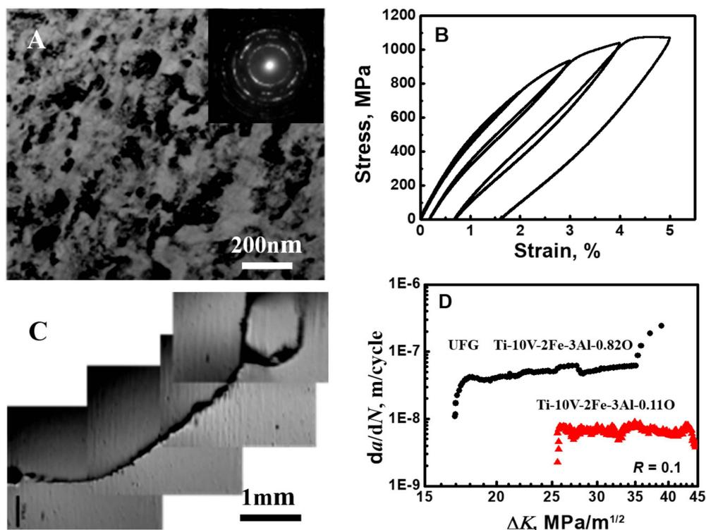
**Figure 7.** Extreme fatigue damage of ultrafine-grained Ti-10V-2Fe-3Al-0.82O alloy with nano-sized  $\alpha$  phase. (A) TEM microstructure and the inset SAD pattern. (B) The nonlinear elasticity. (C) Specimen after three-point bending fatigue test. (D) Fatigue crack growth rate vs. stress intensity factor range.
