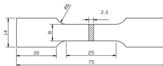
**Figure 1.** Tensile specimen size at room temperature (unit: mm).
