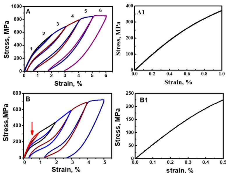
**Figure 4.** Nonlinear elasticity and elastic gradient. (A,B) Cyclic tensile loading and unloading stress–strain curves of the Ti-10V-2Fe-3Al-0.11O alloy and the Ti-10V-2Fe-3Al-0.82O alloy, in which the number on the curve represents the cycle number and the arrow shows the critical stress to induce martensite transformation (MT). (A1,B1) Enlarged stress–strain curves in the low-strain range.
