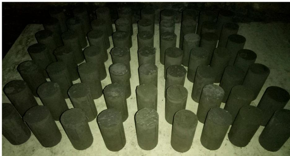
**Figure 2.** The cemented paste backfill (CPB) specimens for the unconfined compressive strength (UCS) test.
