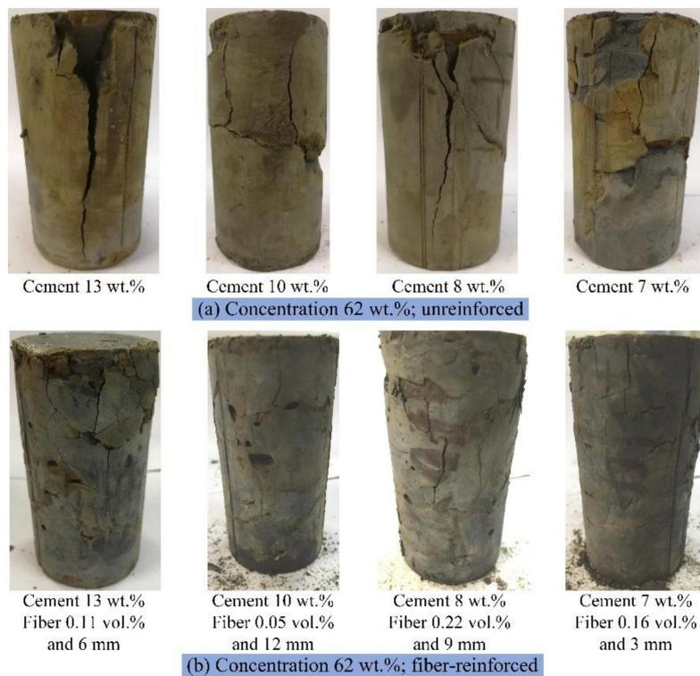
Figure 5. The macroscopic failure modes of the CPB specimens: (a) unreinforced with concentration of 62 wt.%; (b) fiber-reinforced with concentration of 62 wt.%.
