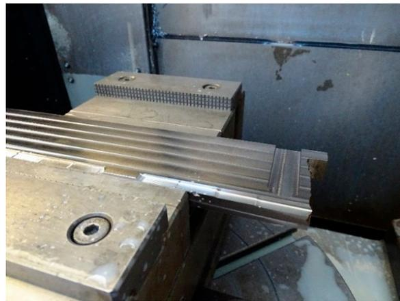
Figure 15. Slot milling across the PAW-WAAM wall.
