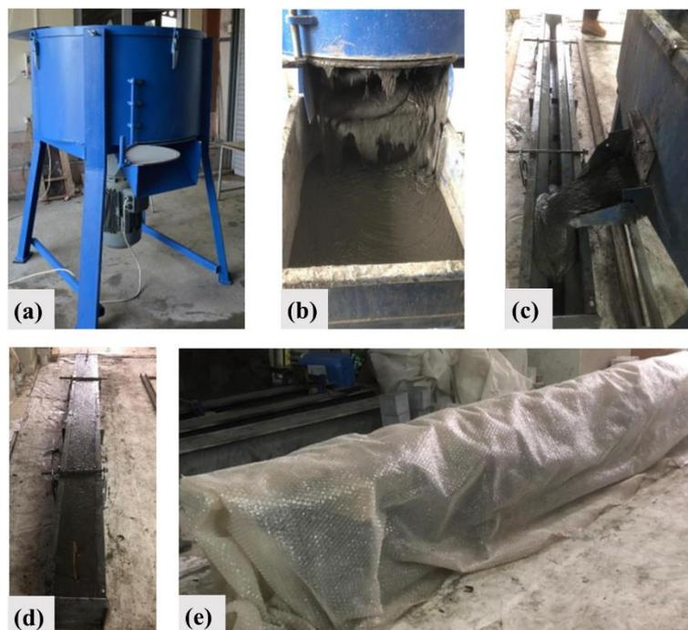
**Figure 1.** (a) Horizontal pan mixer, (b) Pouring, (c) Casting process, (d) After casting, (e) Covered beam.
