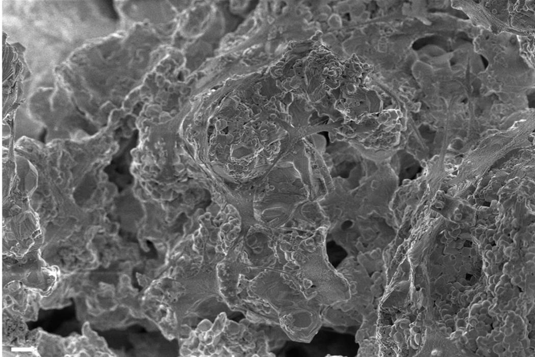
**Figure S3.** SEM images from the direct cytocompatibility test in a lower magnification showing widely spread cells over the BaTiO<sub>3</sub>/HA composite (scale bar: 10  $\mu\text{m}$ ).
