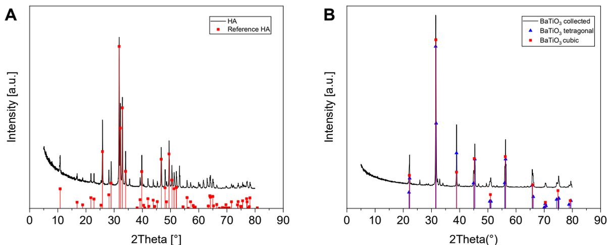
**Figure S1.** Powder diffraction patterns of the ceramic raw materials hydroxyapatite (A) and BaTiO<sub>3</sub> (B). Both patterns are in good agreement with the ICDD reference data 01-076-8436 (ICDD, 2016, hydroxyapatite), 01-081-8524 (ICDD, 2016, BaTiO<sub>3</sub>, tetragonal) and 01-081-8527 (ICDD, 2016, BaTiO<sub>3</sub>, cubic), respectively.
