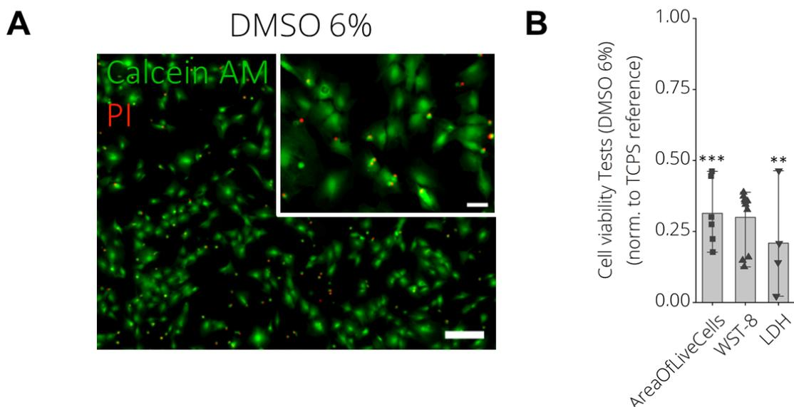
**Figure S2.** Indirect in-vitro cytotoxicity test according to ISO10993 using material eluates. (A) LIVE/DEAD Images of Calcein AM (green, live) and propidium Iodide (red, dead) stained MC3T3-
