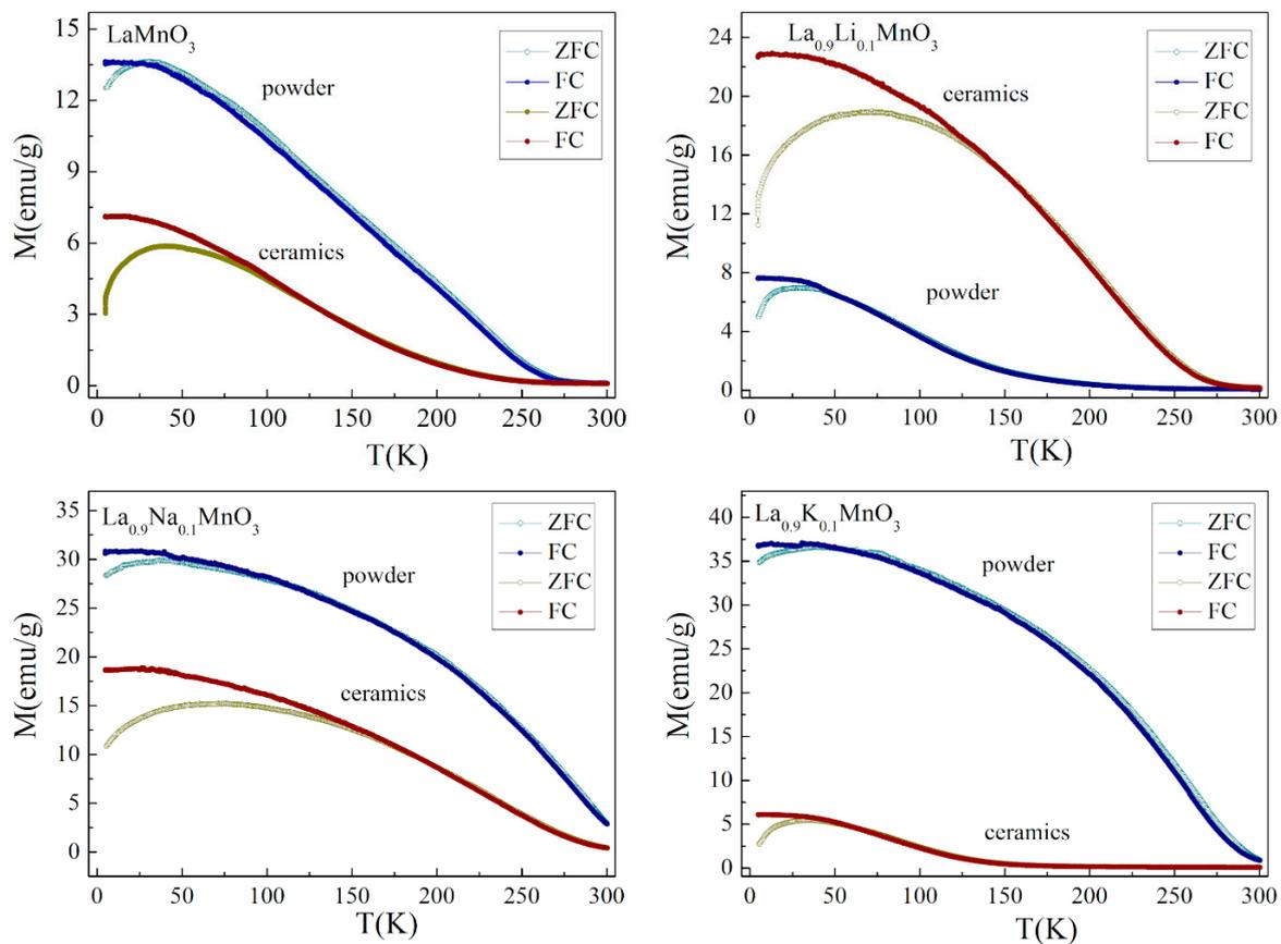
**Figure 7.** Field cooled and zero-field cooled dependencies of magnetization recorded for the  $\text{La}_{0.9}\text{A}_{0.1}\text{MnO}_3$  compounds ( $\text{A} = \text{Na}, \text{Li}, \text{K}$ ) and initial compound  $\text{LaMnO}_3$  in a magnetic field of 1kOe.
