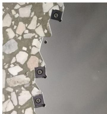
Figure 4. The positioning and clamping mode of inserts and cutter disc.
