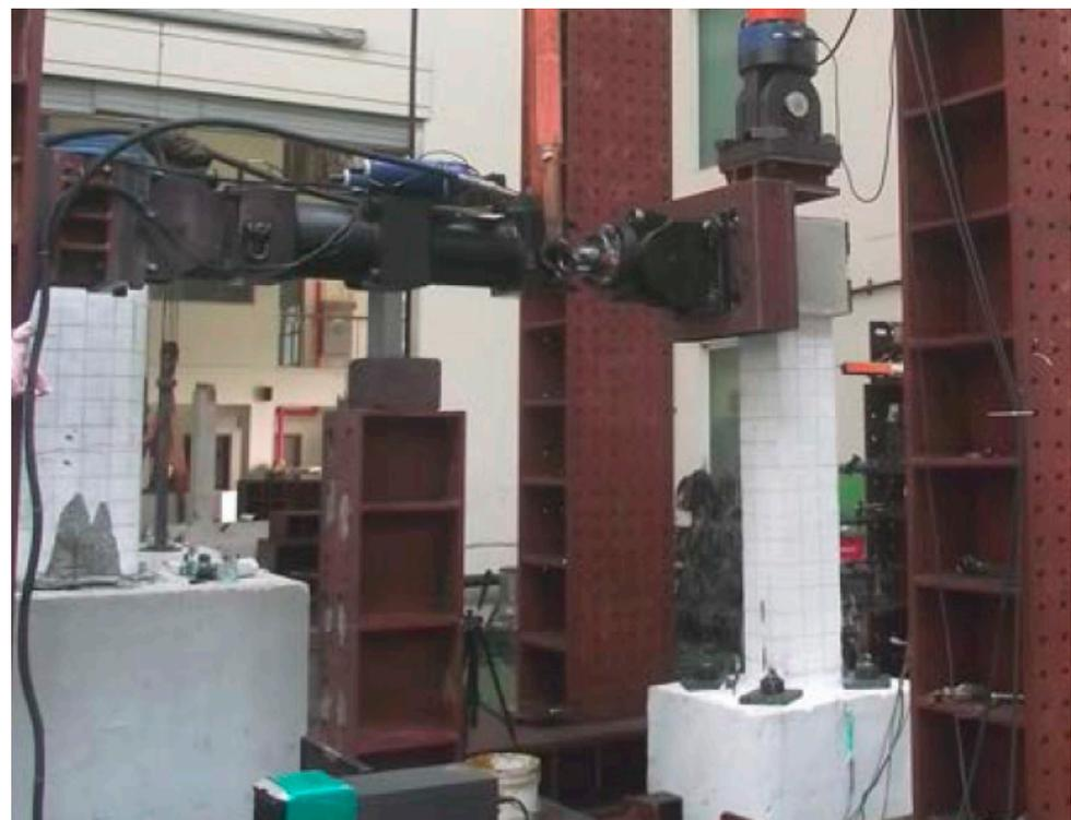
**Figure 5.** Setup for cyclic loading test.
