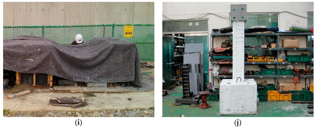
**Figure 4.** Manufacturing process of column specimens (a) Formwork (b) Rebar installation (c) Strain gauges installation (d) ECC mix (e) Mixed ECC (f) Placement of ECC (g) Placement of concrete (h) Finish (i) Curing of specimen (j) Manufactured specimen.
