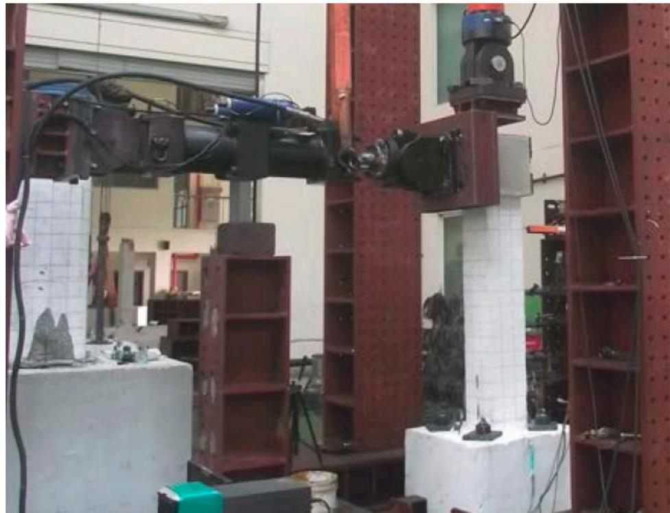
**Figure 5.** Setup for cyclic loading test.
