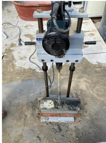
(a) Prismatic specimen vibration compacting
