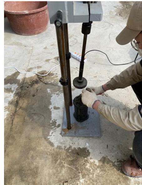
(b) Cylindrical specimen vibration compacting
