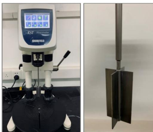
Figure 3. Rheological properties test of cement mortar.
