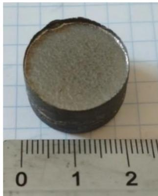
**Figure 2.** Photograph of spark plasma sintered zirconium sample with dimensions  $\text{Ø}20 \times 30$  mm.
