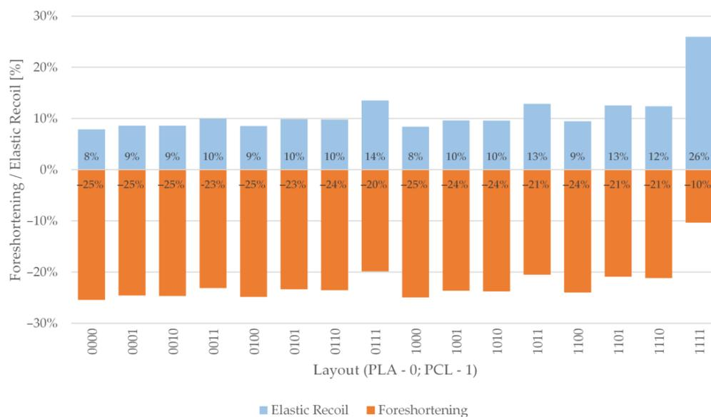
**Figure 10.** Radial elastic recoil and foreshortening results.
