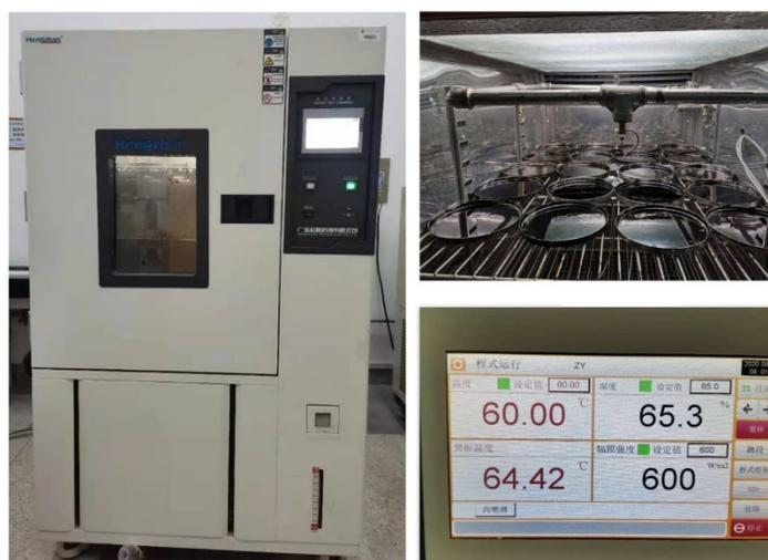
Figure 2. Weather aging apparatus and conditions.
