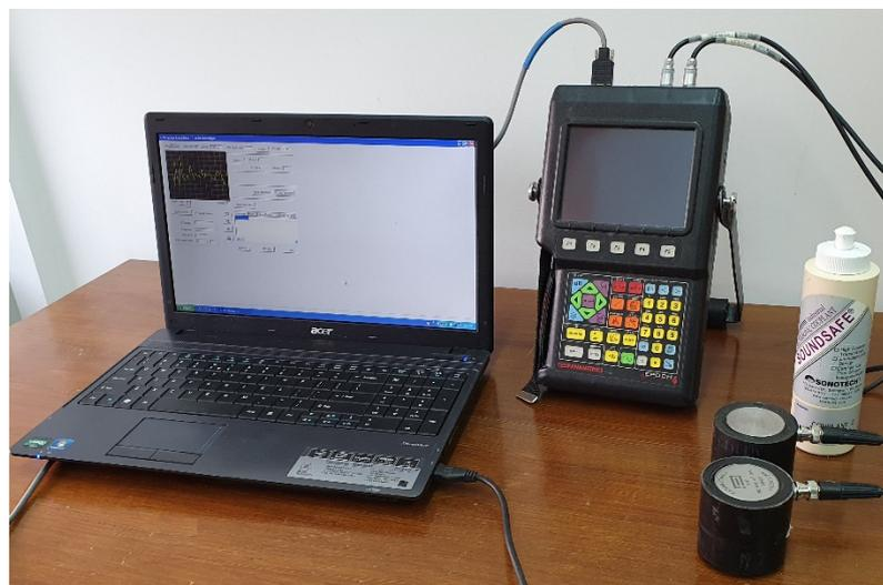
**Figure 3.** The ultrasonic experimental setup used in the study—ultrasonic defectoscope Epoch4, piezoelectric transducers of 100 kHz central frequency and coupling gel (Panametrics NDT-Olympus NDT, Shinjuku, Tokyo, Japan).
