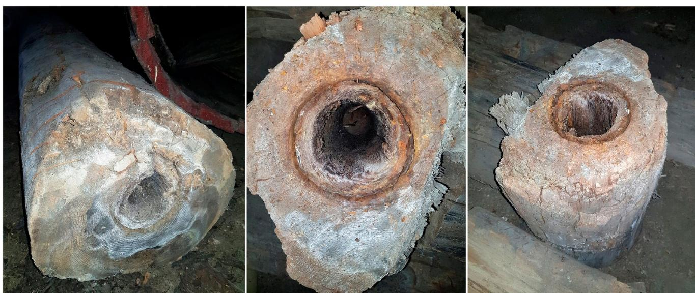
**Figure 2.** Degraded wooden elements of water pipes found during excavations at Bóznicza street in Poznań, Poland.
