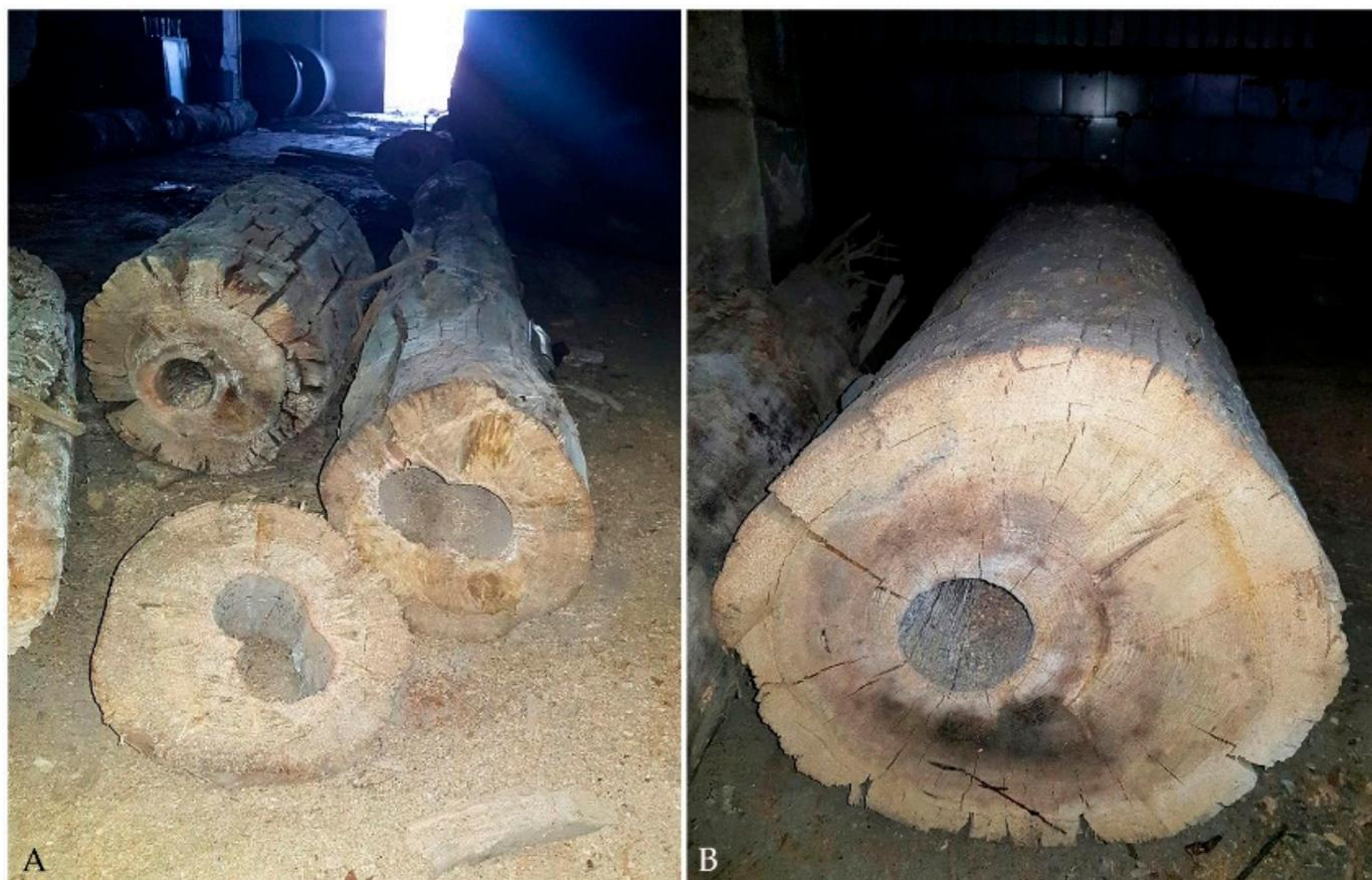
**Figure 1.** Elements of wooden water main excavated at Bóznicza street in Poznań, Poland: (A) more degraded wooden pipes with deep cracks visible in the outer layers; (B) an example of a better-preserved log.
